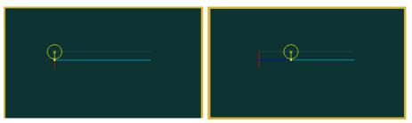
Similarly, the G40 function performs a compensating movement on the first movement when G40 is active.
